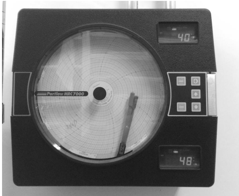
Fig. 3. The Circular Chart Recorder at the Crozier Storage and Conservation Facility of the Cooper Hewitt Smithsonian Design Museum records temperature and humidity measurements on a round chart over a timed interval. Image by Samir Bhowmik.
